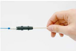
10. Assemble the boot and the cap.
