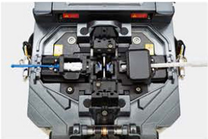
6. Put the ferrule and cable on the V-groove.
