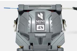
8. Put the spliced connector in the oven, then it will start heating automatically.
