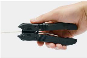
2. Strip the indoor cable with a stripper.
