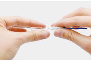
5. Take the fibre protector off from the ferrule.
