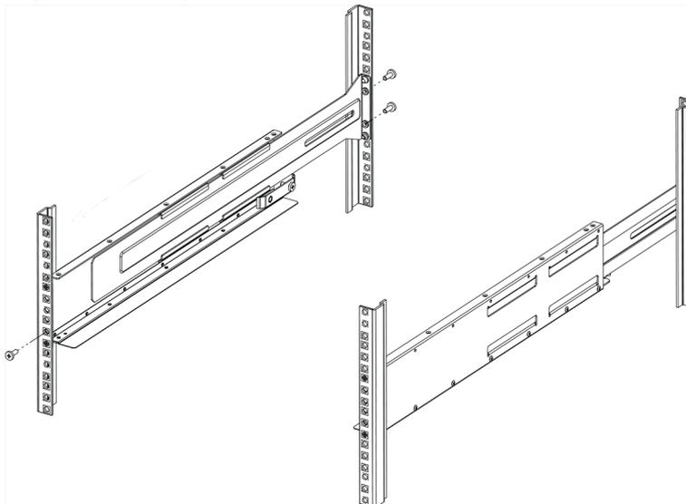
3. Place the back of the unit (the end with the connectors) on the rails.
