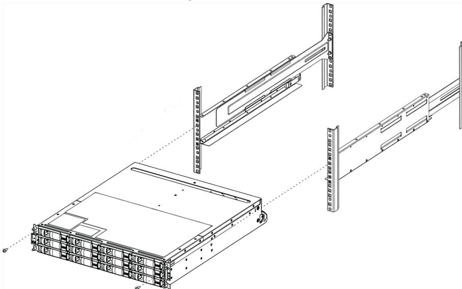
6. Secure the unit to the back of the rails by inserting two M5 screws through the brackets at the unit and the rail kit bracket.
