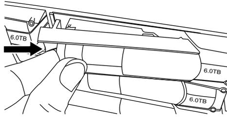
3. Open the cam handle, and slide out the drive slightly.
