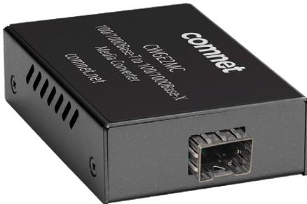
The ComNet CWGE2MC Ethernet media converter series are one-channel Ethernet electrical to optical media converters. These auto-negotiating devices accept a 100/1000 Mbps Ethernet signal and convert this to a 100/1000 BASE-X signal. These devices use either one or two optical fibers, depending upon the selection of either included or sold-separately SFP\* optical module.
