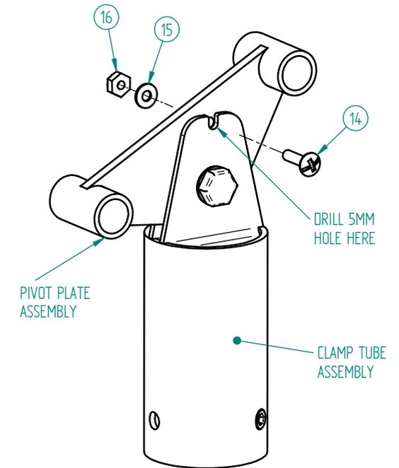
WHEN MOUNTING HEAVY EQUIPMENT AN OPTIONAL LOCKING BOLT (PART 14) MAY BE USED TO SET THE POLE VERTICAL AT ANY INCLINATION.
