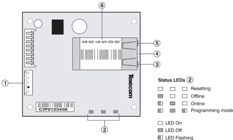
① 5-way harness connection to control panel
